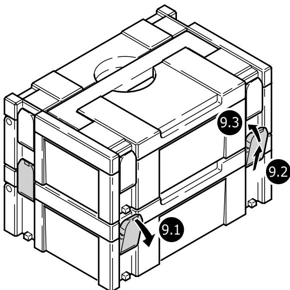
Many Festool products are shipped in a unique system container, called "Systainer". This provides protection and storage for the tool and accessories. The Systainers are stackable and can be interlocked together. They also can be interlocked atop Festool CT dust extractors.
