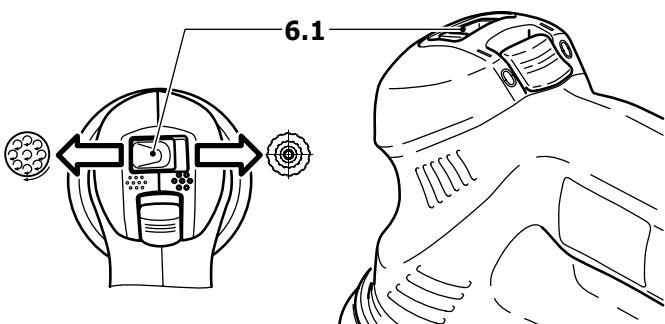
**CAUTION** The change can only be made when the sanding pad is stationary, as the switch is locked in place during operation for safety reasons.
